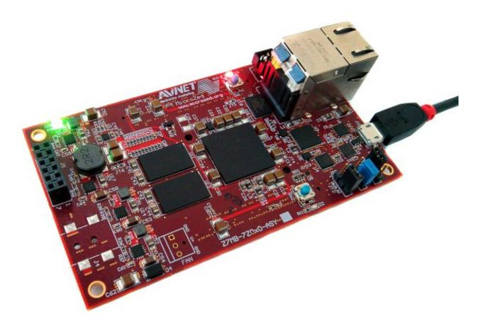
To power-on the board, just connect the mini-USB from PC to Microzed connector. On connector J2 you can also have the serial console, so, during your daily development use, you would just connect your workstation to the board using the mini-USB.
