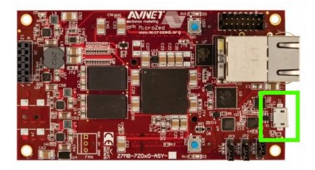
which you can connect, by means of a micro-USB cable, to your personal computer.
